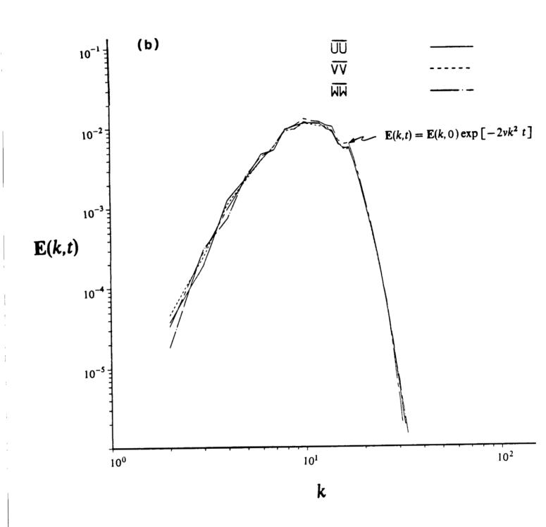
Figure 2. Energy spectrum obtained from a direct numerical simulation of rotating isotropic turbulence: (a) t = 0, (b) t > 0 (K/K<sub>0</sub>  $\stackrel{\circ}{=} 0.1$ ).
