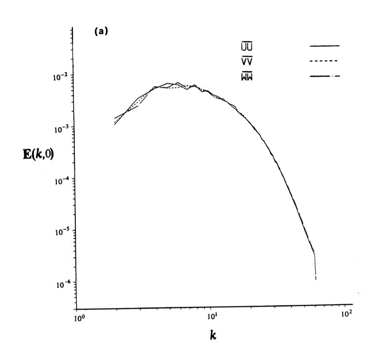
Figure 2. Energy spectrum obtained from a direct numerical simulation of rotating isotropic turbulence: (a) t = 0, (b) t > 0 (K/K<sub>0</sub>  $\stackrel{*}{=} 0.1$ ).
