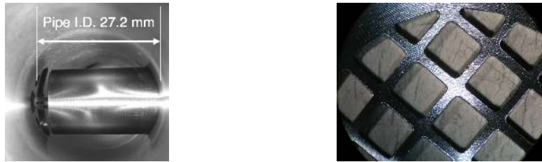
FIG. 6. Left: picture of the removable cylinder in the TSF wind tunnel. The angle between the probe and the axis of the pipe is 17^\circ . Right: picture of the grid.
