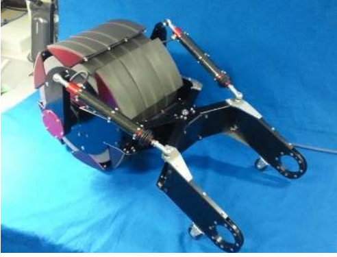
Fig. 8. One trunk module of the ACM-R8. Each module has 3 DOFs: One is for the wheel, and the others are for bending joint in pitch and yaw axes.
