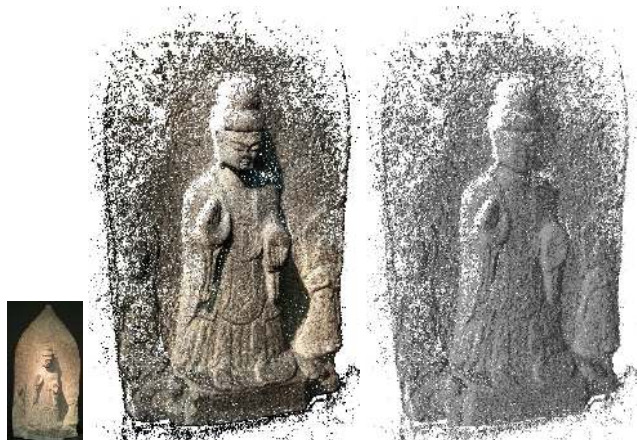
Figure 8. Buddha statue. Rendering of the reconstructed surfel cloud with colors and shading, and a reference image of the object. Note the accurately captured small-scale details.
