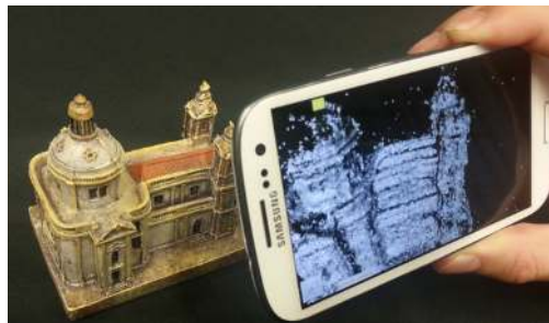
Figure 1. This paper deals with the problem of live 3D reconstruction on mobile phones. The proposed approach allows to obtain 3D models of pleasing quality interactively and entirely on-device.
