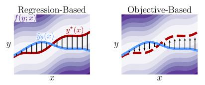
Figure 2.2: Overview of key losses for optimizing the parameters  $\theta$  of the amortization model  $\hat{y}_{\theta}$ . Regression-based losses optimize a distance between the model's prediction  $\hat{y}_{\theta}(x)$  and the ground-truth  $y^{*}(x)$ . Objective-based methods update  $\hat{y}_{\theta}$  using local information of the objective f and without access to the ground-truth solutions  $y^{*}$ .
