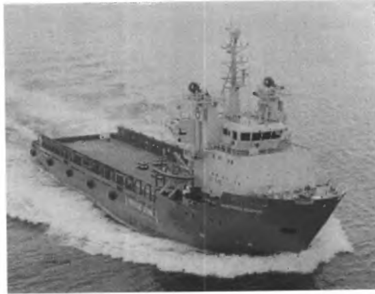
Figure 6. Supply vessel used in the North Sea. Length of ship: 76.2 m.
