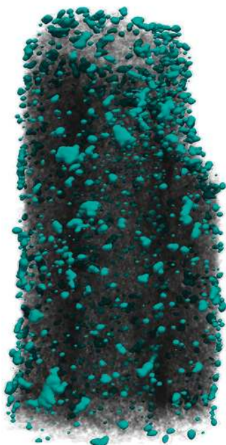
Figure 6: Still image from an animation of platinum particles (turquoise color) on a carbon fiber. The animation is available online in the digital edition of this issue at this web address: https://doi.org/10.1017/S1551929517001213 .
