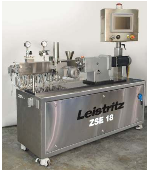
Fig. 18. Downstream side stuffing into the TSE process
