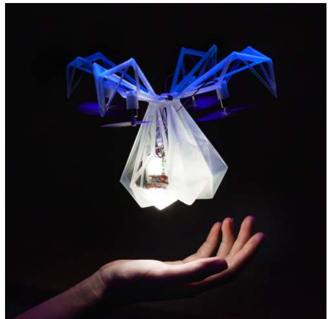
Figure 3. Twinkle’s skin helps convey emotion, protect the propellers, and change its shape and function.
