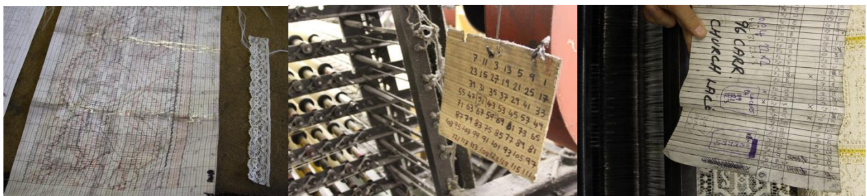
FIGURE 1. A sequence of images showing L-R: ‘draft’ of lace design (schematic diagram of threads); more and less formal ‘figure sheets’ recording the arrangements of machine components needed to produce the pattern. 2013. Photo credit, Julie Botticello. Copyright Nottingham Trent University.
