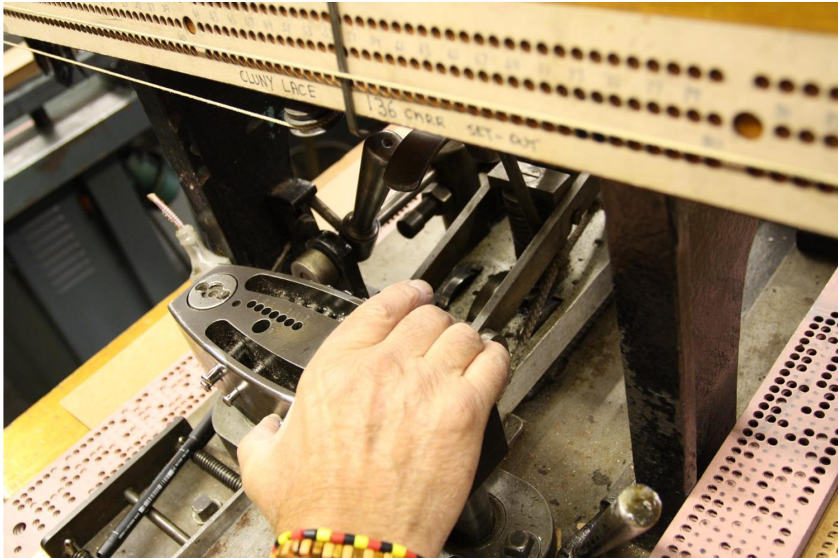
FIGURE 2. The card puncher, Ian Emm, using the card punching machine to transfer the numbers on a figure sheet, to punched cards for the Jacquard mechanism. 2013. Photo credit, Julie Botticello. Copyright Nottingham Trent University.
