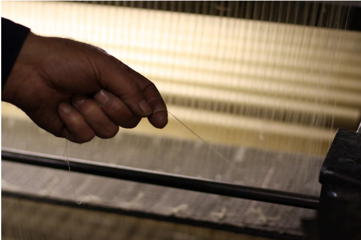
FIGURE 3. A ‘Twisthand’, Ian Palfreman, organizing threads in a Leavers lace machine at Cluny Lace, Ilkeston, 2013. Photo credit, Julie Botticello. Copyright Nottingham Trent University.
