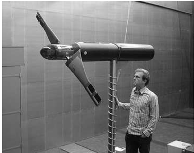
Fig. 1. Photo of the “smart” two-bladed turbine with the trailing-edge flaps. The person standing next to it illustrates the size of the system.
