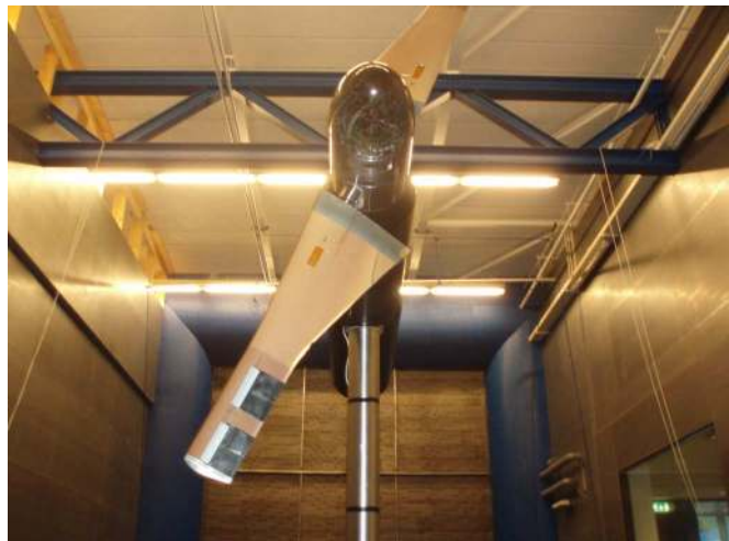
Fig. 2. Photo of the “smart” blade equipped with actuators and sensors.
