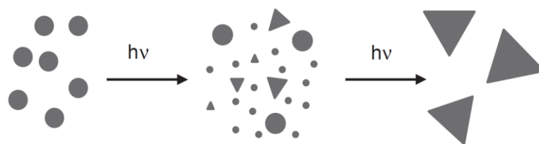
Figure 38: At the early stages of the synthesis, nanoplates and spherical particules are formed. The clusters dissolve and redeposit on the nanotriangles that act as seeds for further growth. From ref.336. Reprinted with permission from AAAS.
