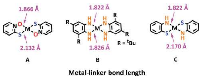
Fig. 3 The bond length of metal-linkers (O, NH, S) in the MX 4 linkage. Selected structures of A, 75 B, 74 and C 76 refer to reported metal-complex small molecules.
