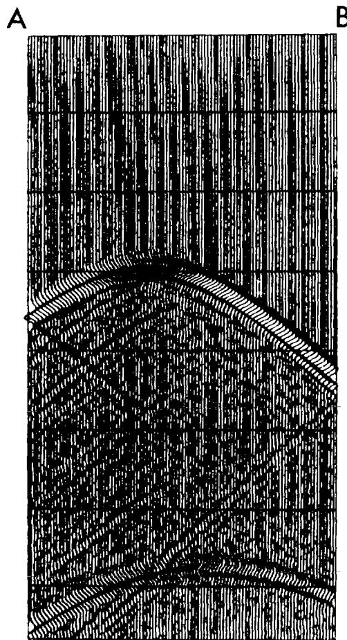
FIG. 7. For the first inversion, eight sources were used (the stars in Figure 8), and each source has been "observed" by 100 receivers in line A-B (one receiver at every other grid point). This figure shows the data corresponding to one of the sources (the star near corner A). The direct wave has been subtracted. A value of \epsilon = 5 percent was used.
