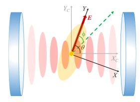
FIG. 1. Scheme of the experimental system. A silica nanosphere levitates on the optical potential created by the light of an optical tweezer, propagating along the Z axis, with the electric field along the Y axis. The nanosphere is positioned on the axis of an optical cavity (which defines the direction  $X_C$ ) in correspondence of a node of the field of a cavity mode. The angle  $\phi$  defines a generic direction in the transverse plane X-Y.
