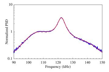
FIG. 6. Heterodyne spectrum (anti-Stokes sideband) normalized to the detection shot noise and with the same shot noise subtracted for the polarization angle that minimizes the effective thermal occupancy in the whole X - Y plane. Red solid line: Fit of the theoretical model.
