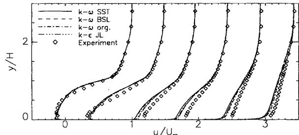
Fig. 8 Velocity profiles for backward-facing step flow at the streamwise locations:  $x/H = 2.0, 4.0, 6.5, 8.0, 14.0$ , and  $32.0$ .
