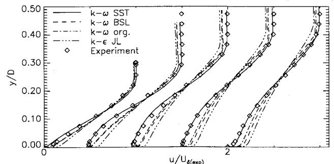
Fig. 4 Velocity profiles for Driver's adverse pressure-gradient flow at  $x/D = -0.091, 0.363, 1.088, 1.633$ , and  $2.177$ .
