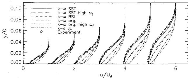
Fig. 9 Velocity profiles on the upper surface of a NACA 4412 airfoil at 13.87 deg angle of attack; streamwise stations  $x/c = 0.675, 0.731, 0.786, 0.842, 0.897$ , and  $0.953$ .
