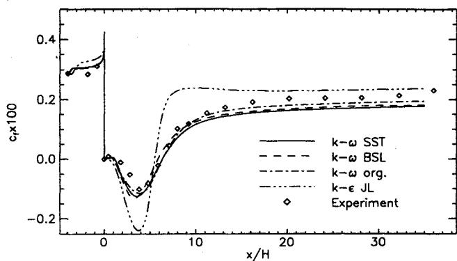
Fig. 7 Wall shear-stress distribution for backward-facing step flow.
