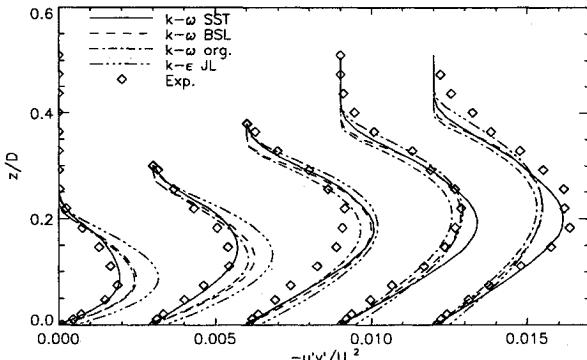
Fig. 5 Turbulent shear-stress profiles for Driver's adverse pressure-gradient flow at  $x/D = -0.091, 0.363, 1.088, 1.633$ , and  $2.177$ .
