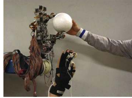
FIGURE 11: Two finger grasping experiment.
