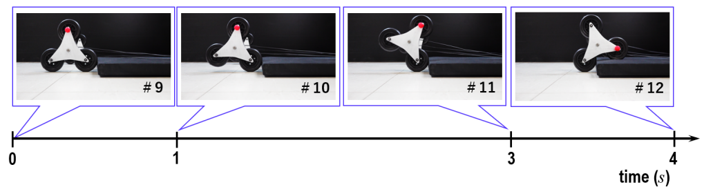
Figure 17. Experimental scenes for comparison analyses where the horizontal direction indicates time over the step-ascending motion according to different wheel types. (a) Case-2: wheel with vertically translated axle; (b) case-5: three-wheel device.
