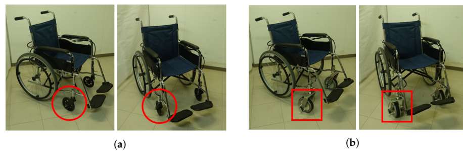
Figure 14. Realization of self-propelled wheelchair using step-ascending prototype. (a) Conventional general wheel; (b) proposed step-ascending wheel.
