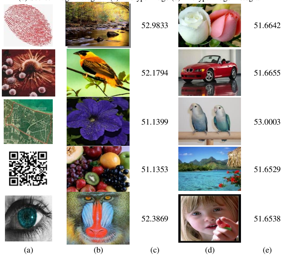
Figure 7. The PSNR of the cover images (Cover1 and Cover2) after hiding operation (a) Secure image (b) Cover image level-1 (c) PSNR of cover1 (d) Cover image level-2 (e) PSNR of cover2
