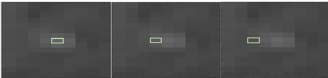
Figure 2. Zoom on the exemplary point in Figure 1. Left: The marked pixel contains the target with the spectrum T as a whole pixel. Center: The marked pixel is a mixed pixel with the spectrum P . Right: The marked pixel is a pure background pixel with the spectrum B .
