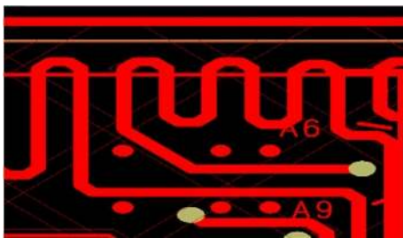
Fig. 15. A6 address line of the "snake-shaped wiring" way
