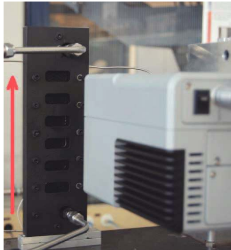
FIG. 4: Photograph of the test section enclosed in PVC frame box and set up on the facility; PHE front view with the arrow showing the flow direction
