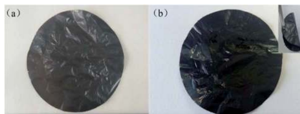
Fig. 2 Digital photographs of the nanocomposite paper (a) before and (b) after hydrothermal reduction (inset: twisted SGP showing good flexibility).
