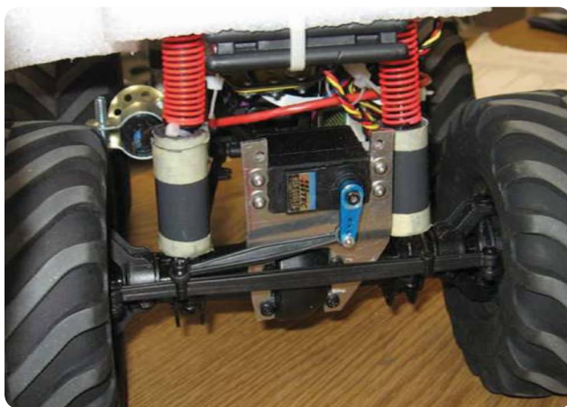
FIGURE 2 Modified high-torque steering servo. The original steering servo has significant compliance and backlash in the drive linkage, which can create instability in the closed-loop system response. A stiffer steering servo mount and a higher performance servo are used to eliminate this problem.
