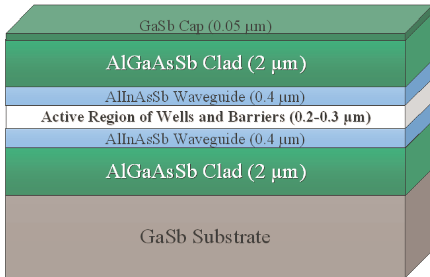
Figure 4. Type I mid-IR laser structure
