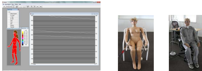
Figure 1. Thermal manikin control screen (left), climate chamber/thermal manikin ‘Monica’ (right).
