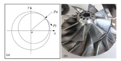
Figure 3. (a) Diagram of rub-impact. (b) Physical diagram of rub-impact.
