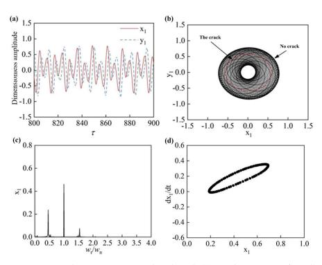
**Figure 11.** Rotor dynamics response under rub-crack: (**a**) time domain curve of impeller displacement change; (**b**) impeller axis locus; (**c**) frequency spectrum of impeller; (**d**) impeller poincare drawing.
