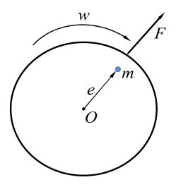
**Figure 2.** Diagram of the rotor unbalanced state. **Note**: *m* is the eccentric mass; *e* is the eccentric distance; *F* is the centrifugal force; *w* is the angular velocity.
