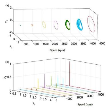
Figure 9. (a) Rotor axis trajectory at different speeds. (b) Rotor spectrum at different speeds.
