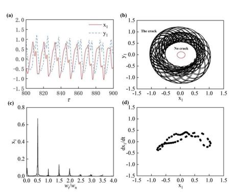
**Figure 10.** Rotor dynamics response under rub-crack: (**a**) time domain curve of impeller displacement change; (**b**) impeller axis locus; (**c**) frequency spectrum of impeller; (**d**) impeller poincare drawing.
