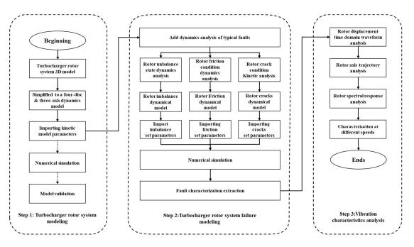
**Figure 4.** Flow chart of typical fault modeling and vibration characteristics study of the turbocharger rotor system.
