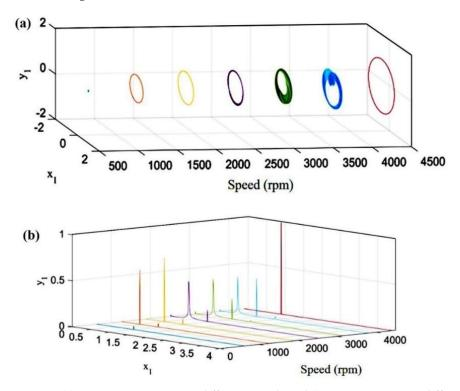
Figure 6. (a) Rotor axis trajectory at different speeds and (b) rotor spectrum at different speeds.
