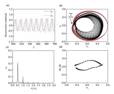
**Figure 8.** Rotor dynamic response under rub-impact: (**a**) time domain curve of impeller displacement change; (**b**) impeller axis locus; (**c**) frequency spectrum of impeller; (**d**) impeller poincare drawing.
