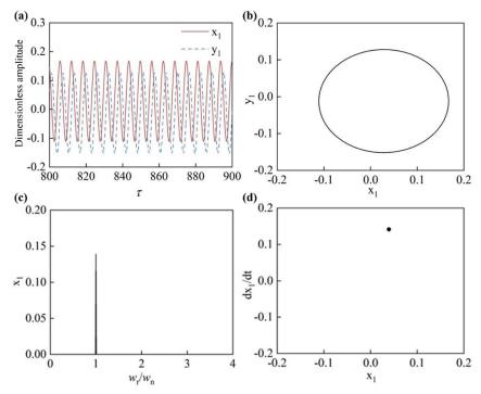
**Figure 5.** Rotor dynamic response under unbalanced conditions: (**a**) time domain curve of impeller displacement change; (**b**) impeller axis locus; (**c**) frequency spectrum of the impeller; (**d**) impeller poincare drawing.
