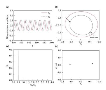
**Figure 7.** Rotor dynamic response under rub-impact: (**a**) time domain curve of impeller displacement change; (**b**) impeller axis locus; (**c**) frequency spectrum of the impeller; (**d**) impeller poincare drawing.
