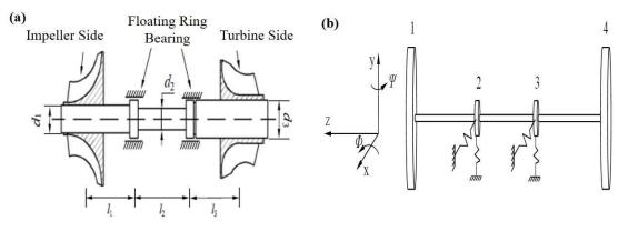
method, and the whole system is simplified to four collector masses of the wheel disc and three shaft segments, as shown in Figure 1.
