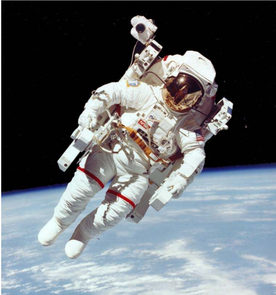
Figure 5. 1984 Bruce McChandless Using a Rocket Pack (Untethered) Called A Manned Maneuvering Unit (Courtesy NASA)
