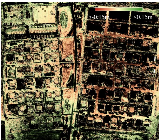
Figure 9: DSM difference between 2nd and 3rd epoch in centimetre range (-15cm to 15cm)
