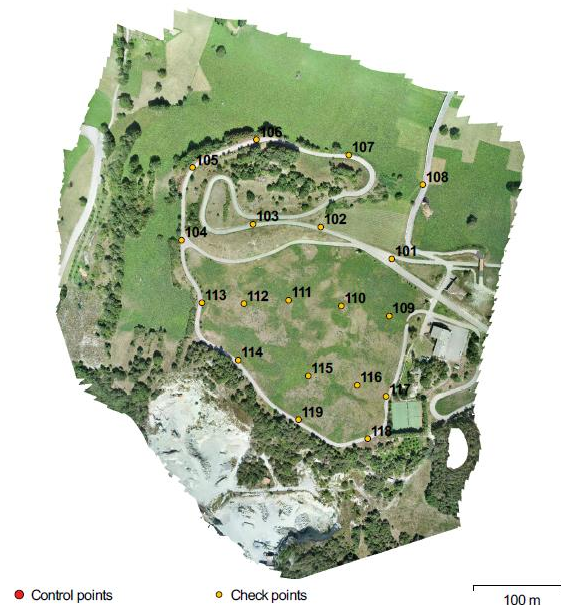
Figure 1. The survey area and the target locations. Most targets act only as check point; some is used as GCP in some tests
