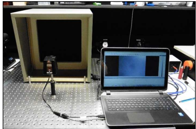
Figure 2. Camera calibration against a blackbody.
