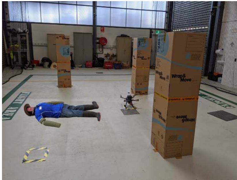
Figure 4. Example of a cluttered indoor environment for UAV Search and Rescue mission. The extent of the free volumetric space area is restricted by randomly placed obstacles. The victim is always lying on the ground and its location is static.
