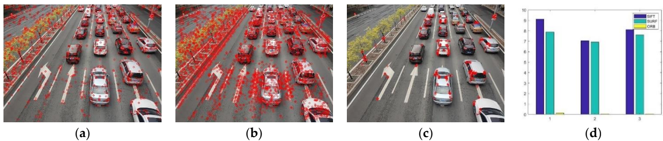
Figure 10. SIFT, SURF, ORB extraction feature point renderings and time-consuming comparison: (a) is the effect of SIFT extraction of feature points; (b) is the effect of SURF extraction of feature points; (c) is the effect of ORB extraction of feature points; (d) is a time-consuming comparison histogram of the three algorithms for extracting feature points.
