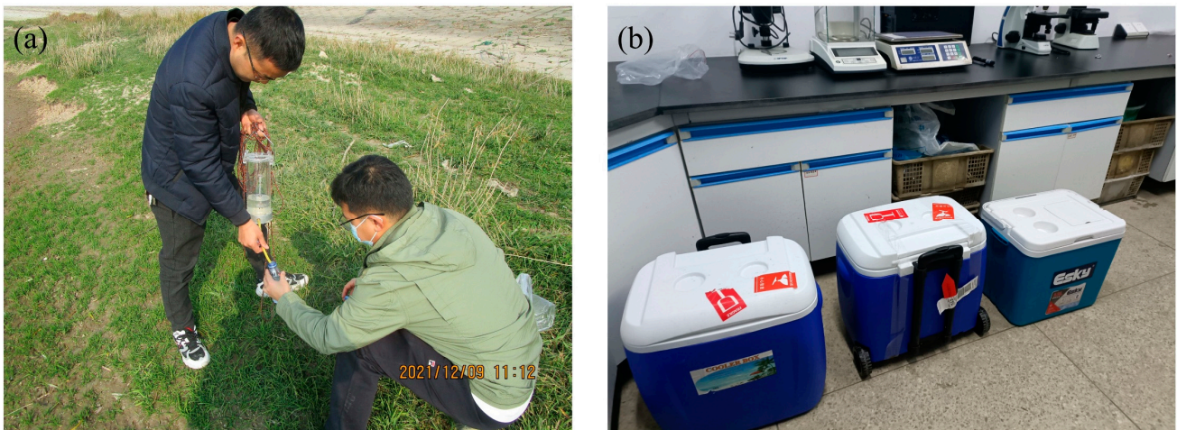
Figure 3. Photographs of field water sample collection and storage: (a) collection of a water sample from the Zhanghe River and (b) water sample storage.
