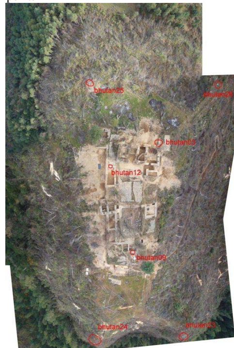
Figure 2: The distribution of ground control points on site.
