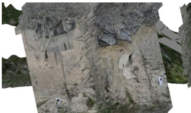
Figure 17. The error in the generation of the point cloud in Context Capture
