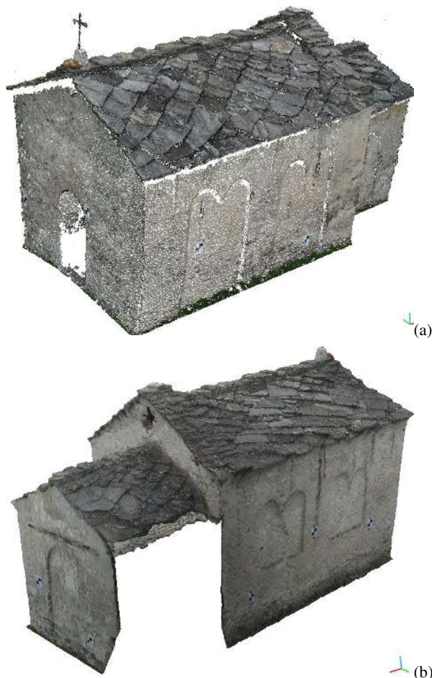
Figure 9. Generated point clouds: software MicMac (a) and ContextCapture (b), which shows the lacking part of façade (covered by the trees).
