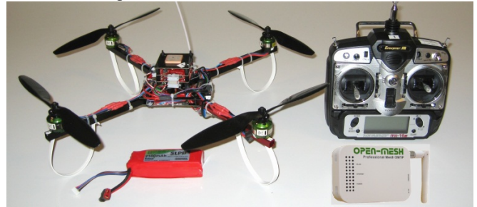
Fig. 1. UAVNet quadcopter & wireless mesh node
