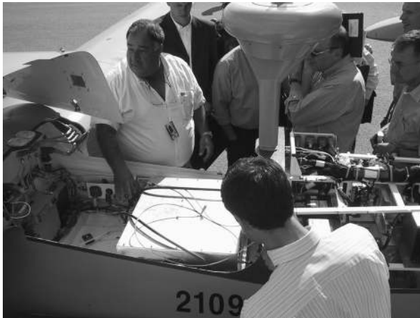
Fig. 5 Payload bay in UAV with CPC (white box)
