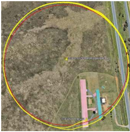
(a) Desired (red) vs Traveled (yellow) trajectory in presence of high latency.
