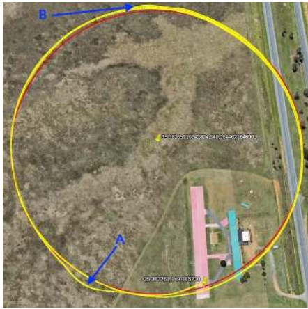
(a) Desired (red) vs Traveled (yellow) trajectory in presence of Packet loss.
