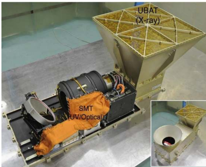
Fig. 1 Flight model of UFFO Burst and Alert Trigger telescope installed on the flight model of UFFO/ Lomonosov without the SMT housing. Inset : UFFO/ Lomonosov with the SMT housing. Each telescope is marked with black text
