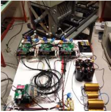
Fig. 6. Multi-three phase rig set-up for testing the uCube
