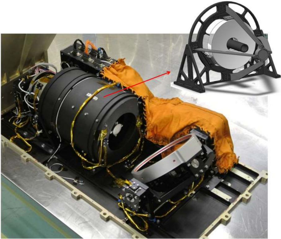
Fig. 11 The integrated SMT system which consists of RC telescope ( upper right ) wrapped by the baffle ( black cylinder ), ICCD and readout ( upper left gray ), and the slewing mirror ( bottom right )
