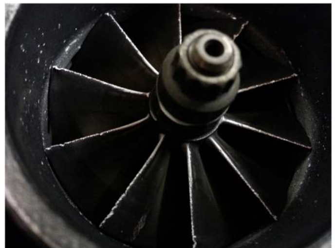
Fig. 31. Turbocharger compressor blade erosion found at the end of testing during Phase 3
