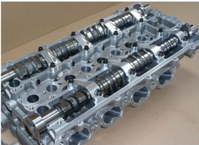
Fig. 3. Cylinder head assembly. Note the fully-machined inlet ports and the twin-lobe 'thumper cams' at the back of the head, providing uneven drive torque for the fast-acting camshaft phasing devices
