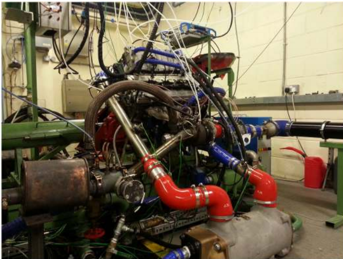
Fig 24. UB200 engine on the test cell at the University of Bath
