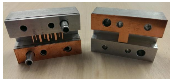
Fig. 27. View of fabricated Filter II.
