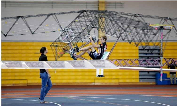
Figure 4. The Gamera Human Powered Helicopter with blade spars, airframe, and cockpit made from wound truss structures
