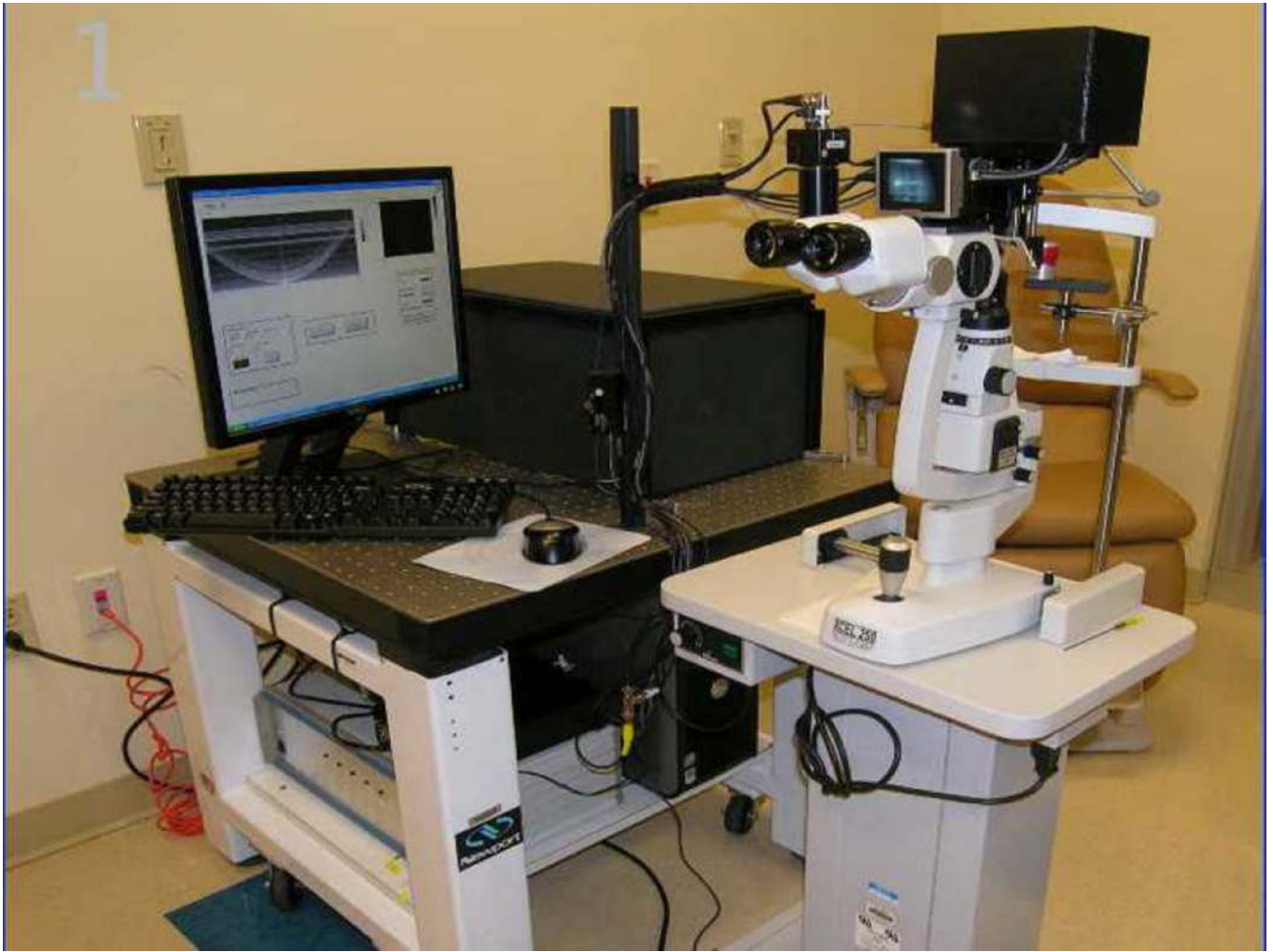
Figure 1. Photograph of the custom-built UHR-OCT device employed at Bascom Palmer Eye Institute, Miami, FL, USA.
