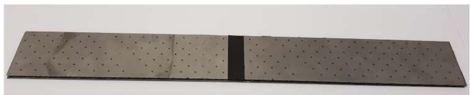
(a) Sandwich panel where the dots on top correspond to the welds.
