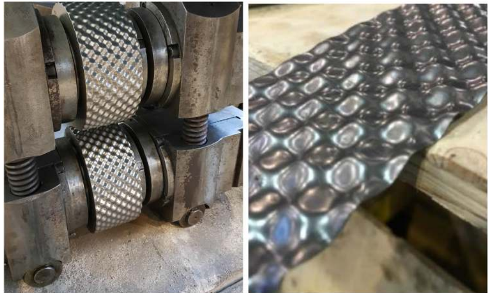
(a) Patterned rolls. Width of rolls are 75 mm and diameter is 180 mm.
