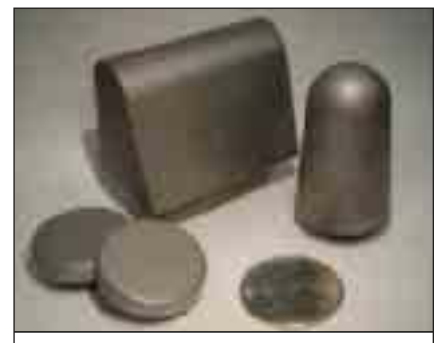
Figure 1. Examples of UHTC Components are shown that have been tested in the NASA Ames Arc Jet facility to evaluate the materials response in a simulated reentry environment. The cone and wedge models are representative of the scale and geometries anticipated for use on UHTC sharp leading-edge vehicles.
