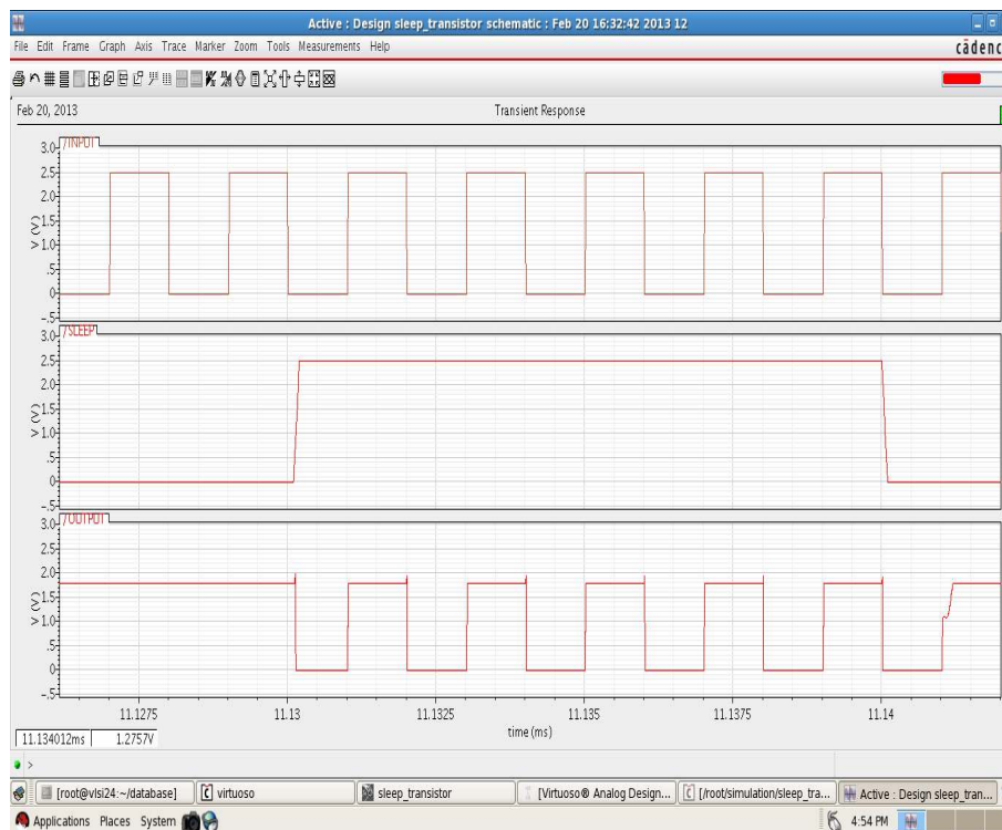
Figure 9. Simulation of leakage feedback dynamic flip-flop [13].
