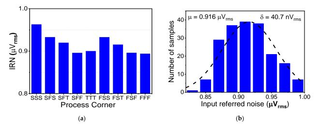
**Figure 15.** The simulation result of (**a**) the CCIA's IRN depending on the process corners and (**b**) the CCIA's input-referred noise.
