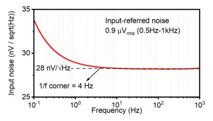
Figure 14. The simulation result of the CCIA's input-referred noise.
