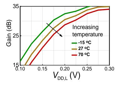
Figure 8. Simulated gain of the SQI stage depending on V<sub>DD,L</sub> and temperature.
