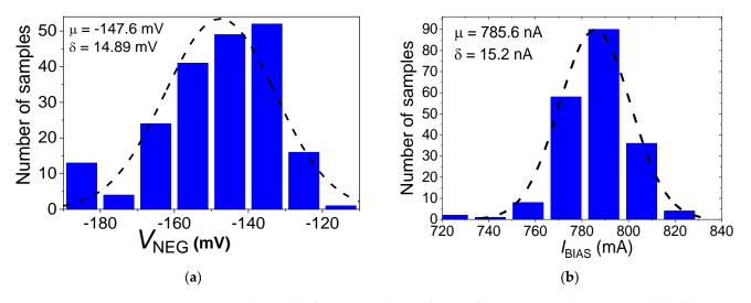
**Figure 7.** The result of Monte Carlo simulation of (**a**) negative voltage  $V_{\text{NEG}}$  (**b**) the bias current of SQI.
