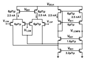
Figure 4. Schematic of CMFB circuit of the SQI.
