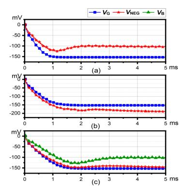
**Figure 6.** Simulated results of the negative voltage generator when the level shifter is powered by (a)  $V_{\text{NEG}}$ , (b)  $V_{\text{G}}$ , (c)  $V_{\text{B}}$ .
