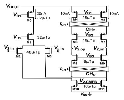
Figure 9. The schematic of the FC amp circuit.
