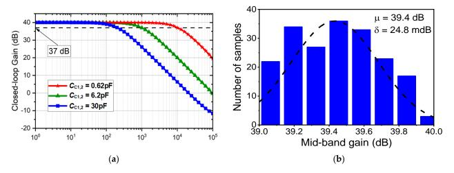
**Figure 12.** (**a**) The CCIA's variable bandwidth of the transfer function, (**b**) CCIA's the Monte Carlo Simulation of the middle-band gain.
