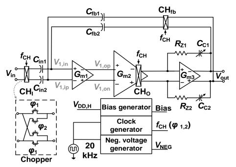
while maintaining bandwidth, Miller compensation capacitors  $C_{C1,2}$  and resistors  $R_{Z1,2}$  are added to the last stage feedback loop.
