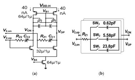
**Figure 10.** (a) The schematic of CS amp circuit, (b) the schematic of phase margin compensation circuit.
