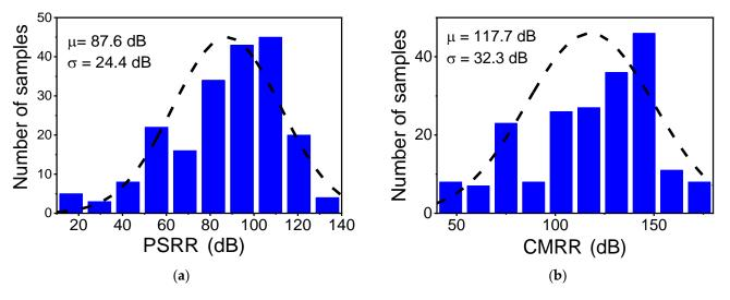
Figure 13. The Monte Carlo simulation result of (a) the CCIA's PSRR, (b) the CCIA's CMRR.
